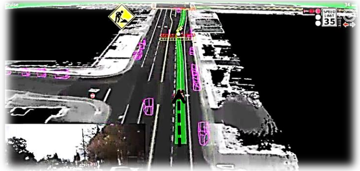
Diagram to show the path of a Google Self-Drive Car as it maps out the objects that are surrounding it.
