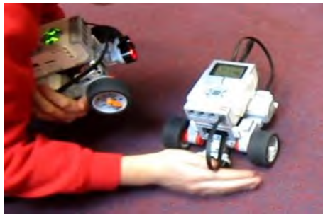
Playing with a Lego EV3 robot with an ultrasonic sensor. Put your hand out and the motors stop. Put a repeat on and it keeps doing it.
